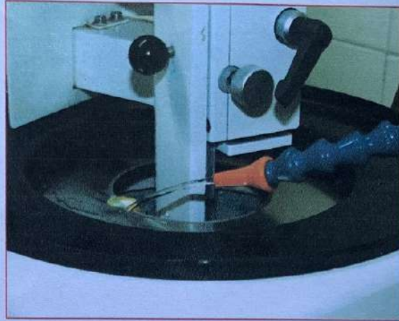
Fig: Showing Hard Tissue Microtome and Cutting of tooth Sections
